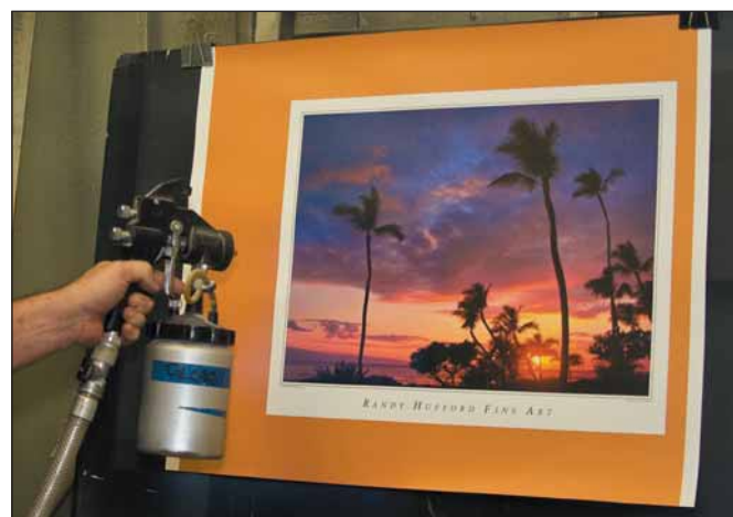
A coating of PremierArt Eco Print Shield is applied to a canvas with a spray gun.
