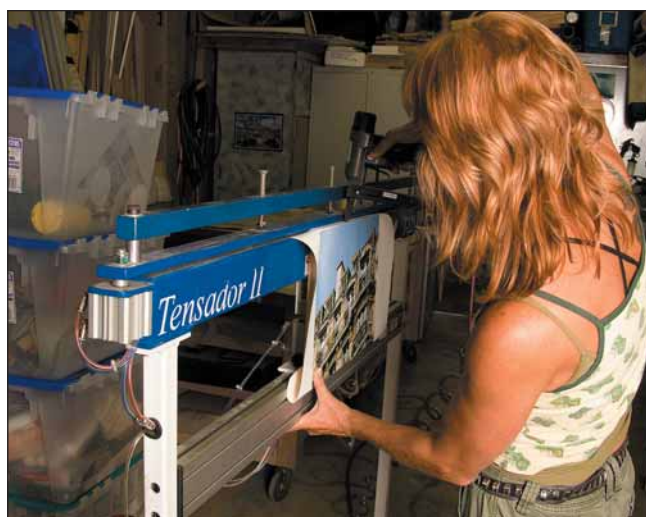
After coating, the canvas should be stretched. For production work, a canvas stretching machine such as the Tensador II makes the process much faster than stretching by hand.
