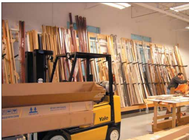
Vertical moulding storage
