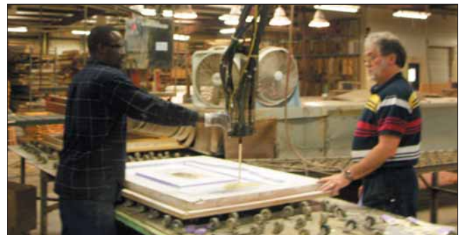
The polymer is poured into a mold at the Foamtech factory. Each mold can be used to produce 60 to 75 reproduction frames each before wearing down.
