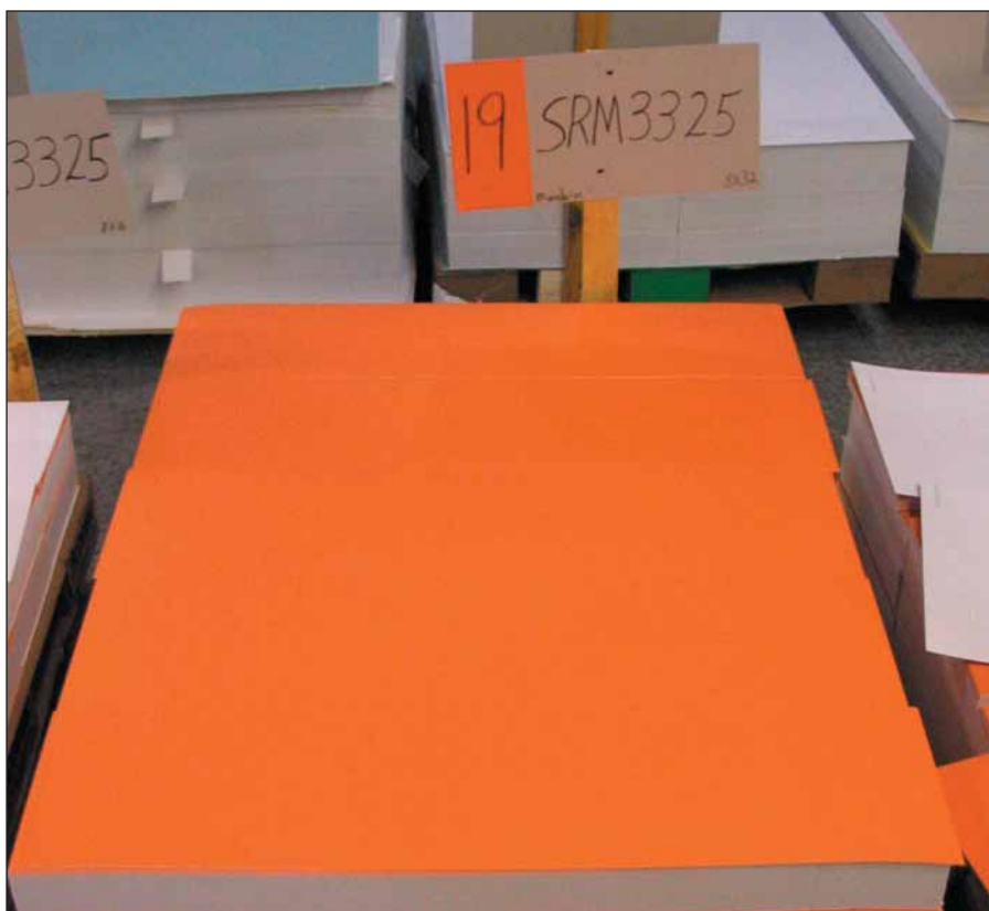
Color codes and short numbers are used to indicate mats and other materials needed for a job. This makes it easy for a worker to pull the right materials without error.
