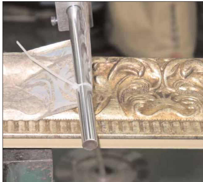
Foil is applied to polystyrene moulding at the MyMoulding factory.
