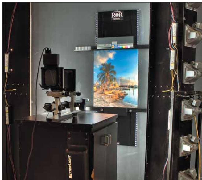
This direct digital scanning set-up includes a custom-built 5000° K light bank, an R&R copy wall, and a 4x5 camera on a rolling back with a BetterLight scan back.
