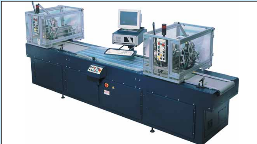
The ITW AMP High Speed Tab Robot can install tabs in 60 frames a minute for frame sizes of 5"x7" to 20"x20" and can be linked to a matching Frame Assembly Robot.
