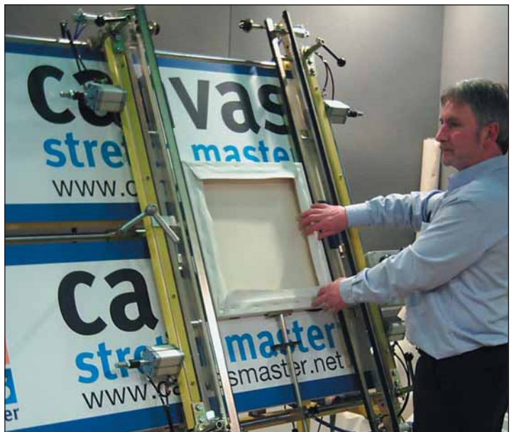
A salesperson demonstrated how to stretch a gessoed canvas on the Canvas Stretch Master.
