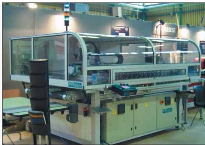
Cassese showed a variety of machines including an automatic frame backing machine for installing Flexipoints and U-shaped staples.
