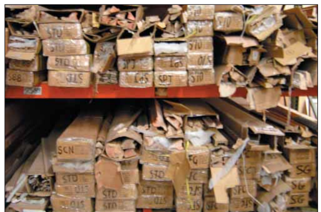
Proper moulding storage (above) helps minimize damage while improper storage (below) can lead to increased damage.
