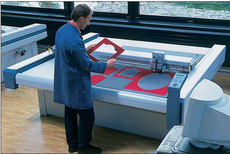
The Zund 1600 is a high-end machine featuring a vacuum table that can make bevels, straight cuts, and French lines with one cutting head.
