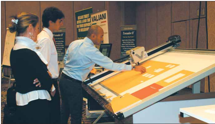
The Plus-is from Valiani is an electronic automated CMC designed for round-the-clock high-speed cutting, with rapid blade change and a mat stylus for French lines.
