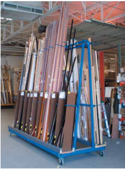
For orders that arrive in smaller, varied batches, rolling vertical storage can be loaded and moved close to the production area (left). In comparison, for larger runs, centralized storage (right) can be located close to loading docks, with horizontal storage that includes moulding and mixed items like art or matboard.
