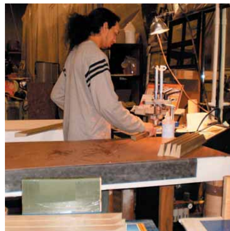
Joining operations can be supplied from rolling carts design for either small or large runs. In this case, the same operator cuts and joins a small batch order. The workflow is switched to an in-line set-up for longer production runs.
