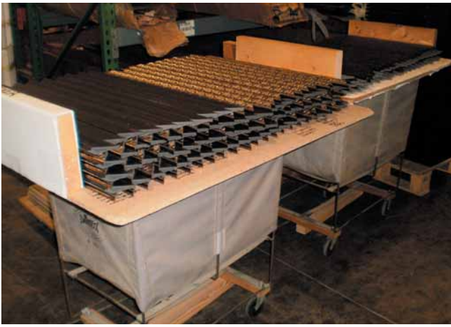
Rolling carts can be used on in-line production of larger orders, as these are used to move quantities of cut moulding to a joining station.
