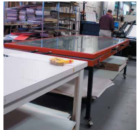
When mounting smaller batches of artwork, a heated vacuum press on wheels can be moved into position. A laminator could also be wheeled into the same position for jobs that call for that kind of mounting.
