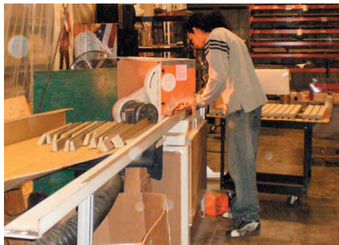
In this in-line set-up, moulding is cut for frames and then placed on carts that travel only 10 feet to the joiner.
