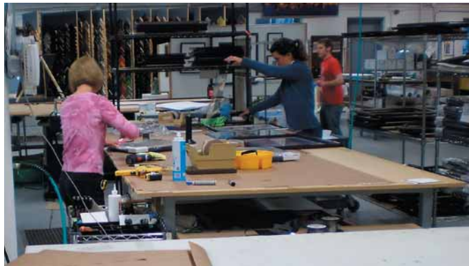
This fitting cell works is designed for producing quantities of framed art of similar sizes as well as for joining a variety of different framing products. Finished pieces are placed on carts for delivery to the shipping department.
