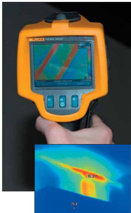
Thermal imaging done during an energy audit can reveal areas that show where non-conditioned air is coming in and where conditioned is leaking out of a facility.
