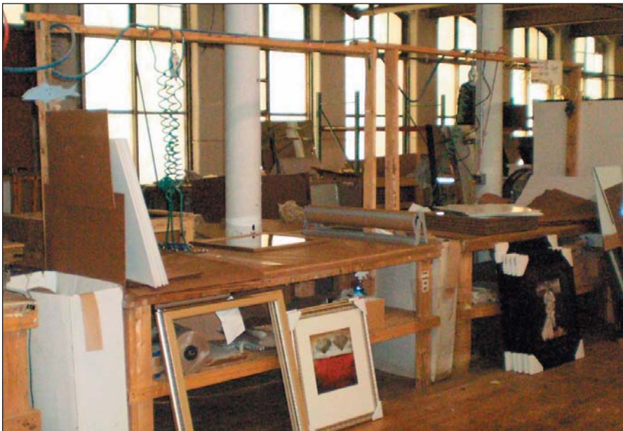
A basic workstation can include an overhead bar for hanging tools and air lines and a shelf for storage of other tools below the main work surface.
