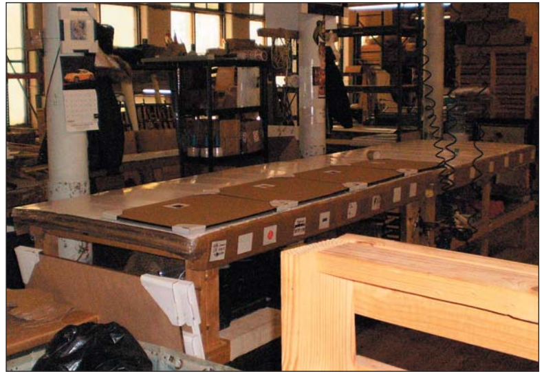
A worktable used for adding protective corners and packaging is similar to a fitting station but without the need for an overhead rail for tools. Padding on the surface of the table helps protect finished frames as they are packaged.
