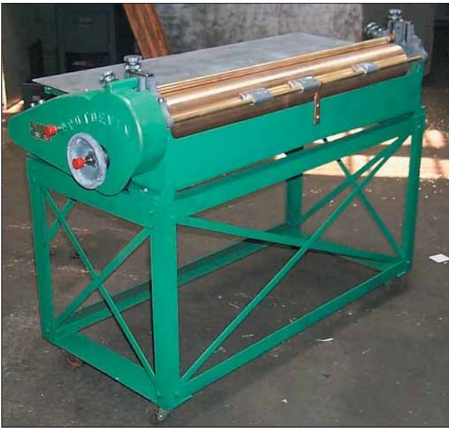
Roller gluers, along with companion rotary presses, can speed up mounting when doing a large quantity of backing boards.
