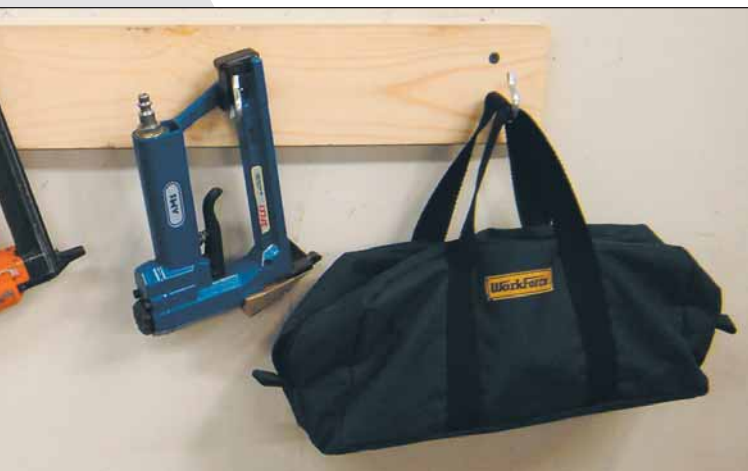
Work stations should have a place for each tool, with no toolboxes or drawers to interfere with visibility or requiring unnecessary motion to open and close.
