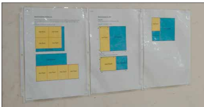
Wall charts at workstations should clearly show standard procedures, such as this one showing a facility's preferred ways to cut mats.
