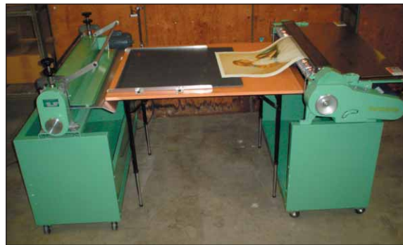
The Potdevin NTZ Gluer and Rotary Press are a popular combination used by production framers to wet mount prints.
