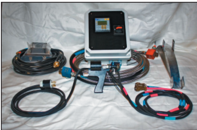
A foam-in-place system uses a two-part polyurethane foam that is sprayed or poured into plastic pouches or bags. This expands, filling voids in a box and provides cushioning.
