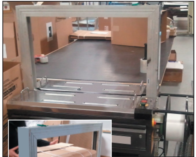
A bridge-type strapping machine is usually automatic and therefore slightly faster than a semi-automatic one.
