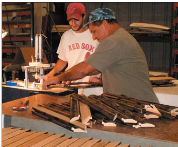
Learning to run a computerized joining machine requires an operator to find stored profiles in a computer as well as making good corner joints.
