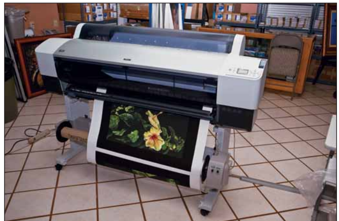
An Epson 9880 digital printer has excellent color reproduction. It is shown here with an optional take up for printing continuous rolls of prints.
