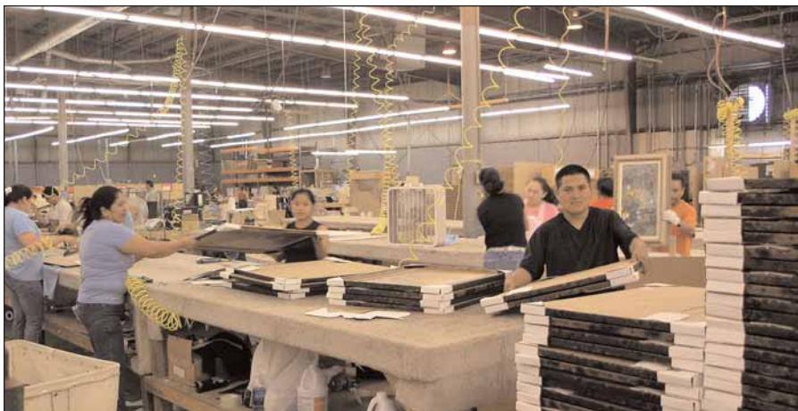
Workers are placed at the beginning and end of a production line, essentially setting the pace at an OEM factory. Floaters such as the man on the right loading the frames assist with the busiest stations.
